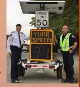
Research has shown that Speed Reader Boards do work. Over 70% of drivers travelling 10km/hr over the speed limit slow down when they observed a speed reader board. Sometimes our drivers just need a little friendly reminder to slow down and make smarter driving decisions.
